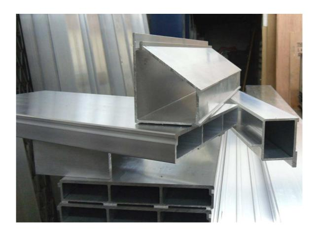
Extrusion is a manufacturing process (thermo) mechanic whereby a compressed material is forced through a channel having the form of the part to be obtained forming a continuously long product (tube, pipe, profiled) and flat (plate, sheet, film).
